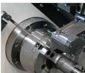
Chuck Air Blow (Upper Chuck)
