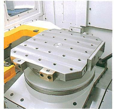
● Full 4th axis rotary table
