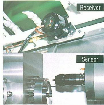
● Automatic measurement (probe sensor)
