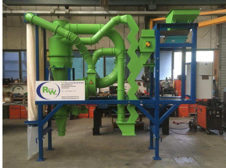
Example: Separation with semi mobile Zig Zag Sifter Plant ZZS 200-15-SM
