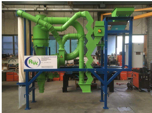
Example: Separation on semi mobile zig zag sifter plant ZZS 200-15-SM
