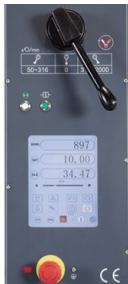
Drill press 2.0 - all functions on a rugged touchscreen
