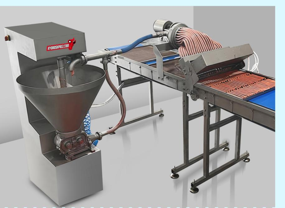
Semi-automatic system for molding thick meat into cylinders and flat strips without alginate casings. Ensures a complete meat forming cycle. Equipped with trolleys and trays for transport and supported by drying chambers
