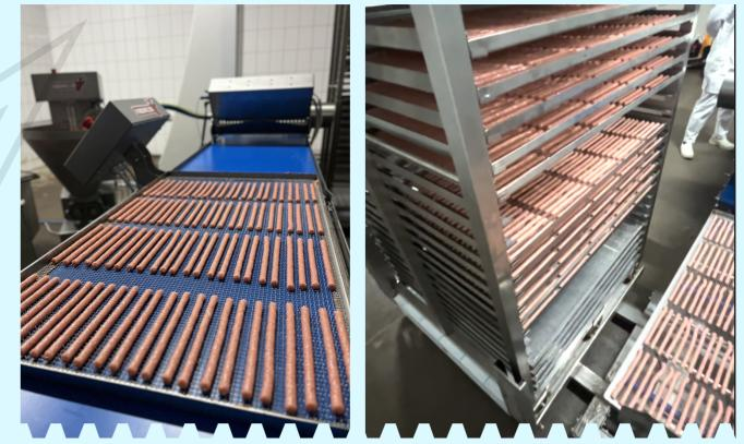
Fully robotic system for producing meat and fish stick snacks, meat strips, jerky, and pet sticks without alginate casing. Designed for thick masses, minimal operator involvement, shaping cycle, supplied with trays and drying chambers.
